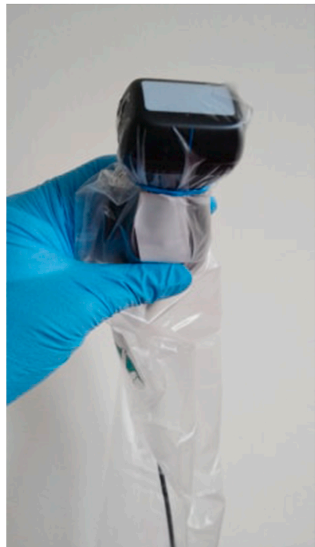
Fig. 1a. Ultrasound transducer in a foil sleeve protecting it against contamination.
