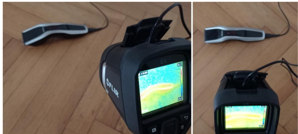
Figure 12. Thermographic measurements for the BLDC motor (clipper HC5440/80).
