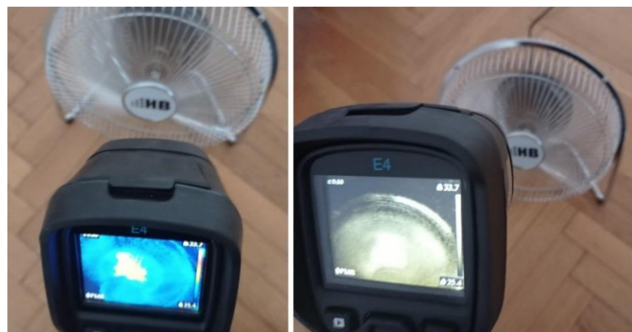
Figure 11. Thermographic measurements for the BLDC motor (fan).
