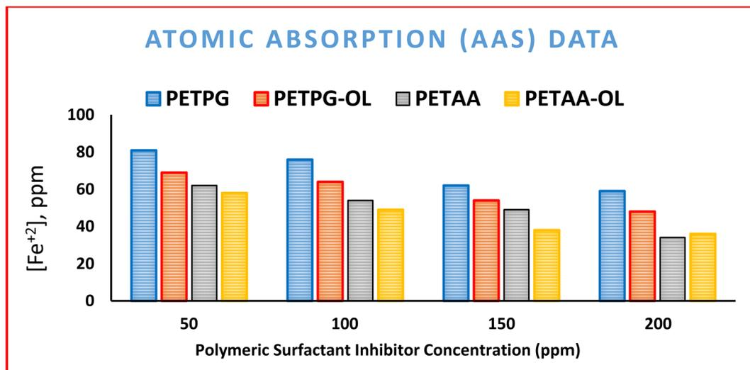
Fig. 8 Effect of four prepared polymeric surfactant inhibitor concentrations on ferrous ion concentration  $[\text{Fe}^{2+}]$  in the presence of 3.5% NaCl solution, as measured by atomic absorption spectroscopy (AAS).
