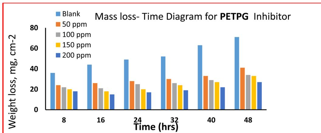
Fig. 6 Weight loss of steel in 3.5% NaCl over time with and without the presence of a prepared polymeric surfactant (PETPG) inhibitor derived from plastic waste.
