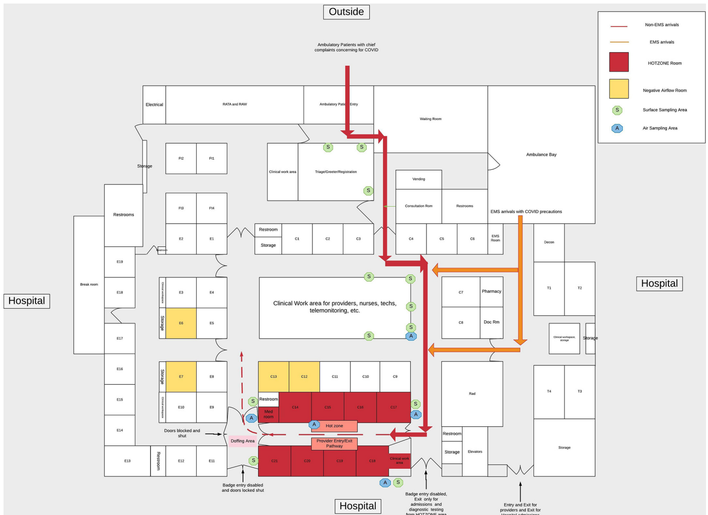
Fig. 1. Diagram of ED representing patient pathways to hot zone and specified air and surface sampling sites.
