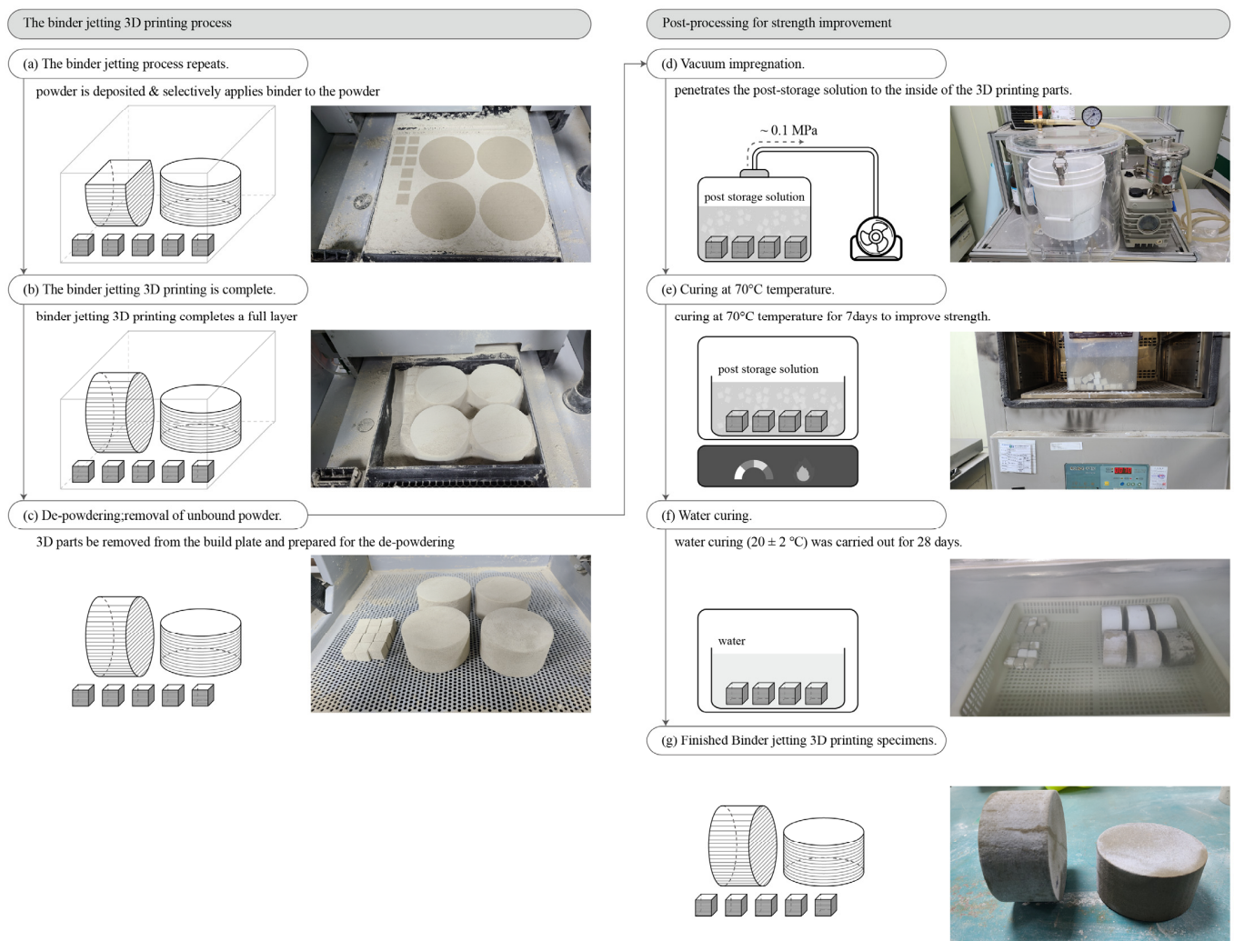
Figure 2. Binder jetting 3D printing process and postprocessing for strength improvement: (a) The binder jetting process repeats, (b) The binder jetting 3D printing is complete, (c) De-powdering removal of unbound powder, (d) Vacuum impregnation, (e) Curing at 70 °C temperature, (f) Water curing, and (g) Finished Binder jetting 3D printing specimen.
