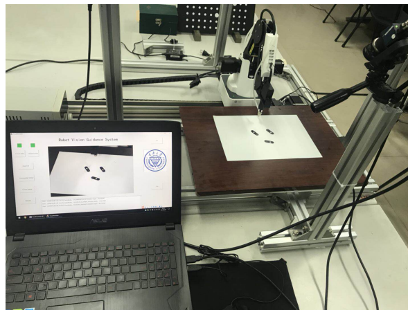
Figure 14. Automatic sorting system with machine vision.
