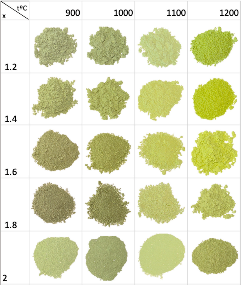
Fig. 18. The digital images of the samples produced from Zn_{2-x}Ni_xSiO_4 compositions with x ranging from 1.2 up to 2.0 by the modified approach to the precipitation method and then heated at different temperatures from 900 up to 1200 °C.
