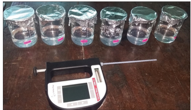
Figure 3: Electronic density meter (DMA 35) for measuring the samples densities
