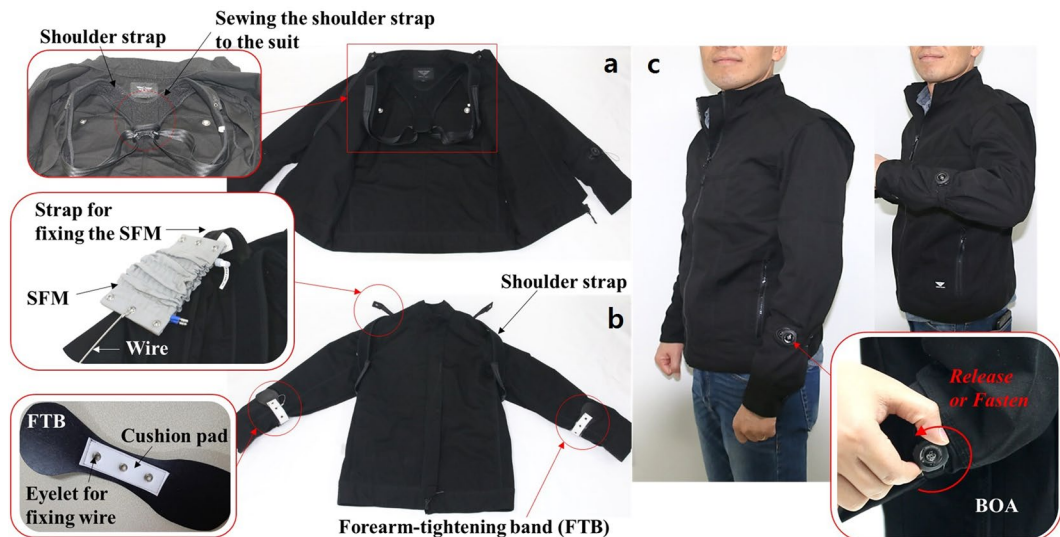
Figure 3. Fabricated STWR: (a) Interior of the STWR. On the back part, the shoulder strap is sewn and fixed. (b) The STWR is turned inside out to show the configuration inside the STWR. By attaching additional straps to the fixed shoulder strap, the SFM is fixed. An FTB on the lower sleeve is connected to the SFM via wires. (c) A human wearing the STWR. The dial of the BOA located on the forearm is turned to fasten or release the FTB on lower sleeve. Even with the FTB fixed, the arm-bending motion is comfortable and activities can be freely performed.
