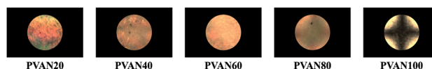
Fig. 8 Conoscopic POM images of the LC cells made from PVAN# films on PET (polyethylene terephthalate) substrates according to the molar content of vanillyl butyl ether moiety.
