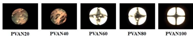
Fig. 5 POM images of the LC cells made from PVAN# (PVAN20, PVAN40, PVAN60, PVAN80, and PVAN100) films.
