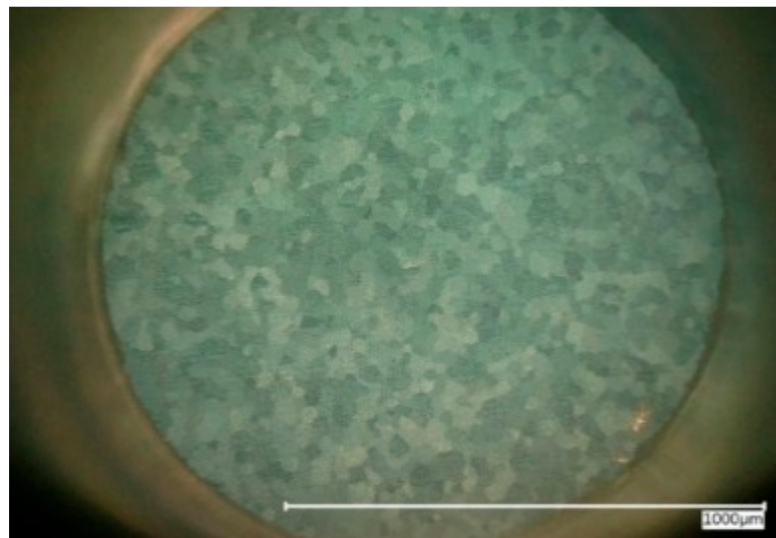
Figure 3. The cp Mg surface as seen through video-optical-electrochemical cell, polarized lighting.
