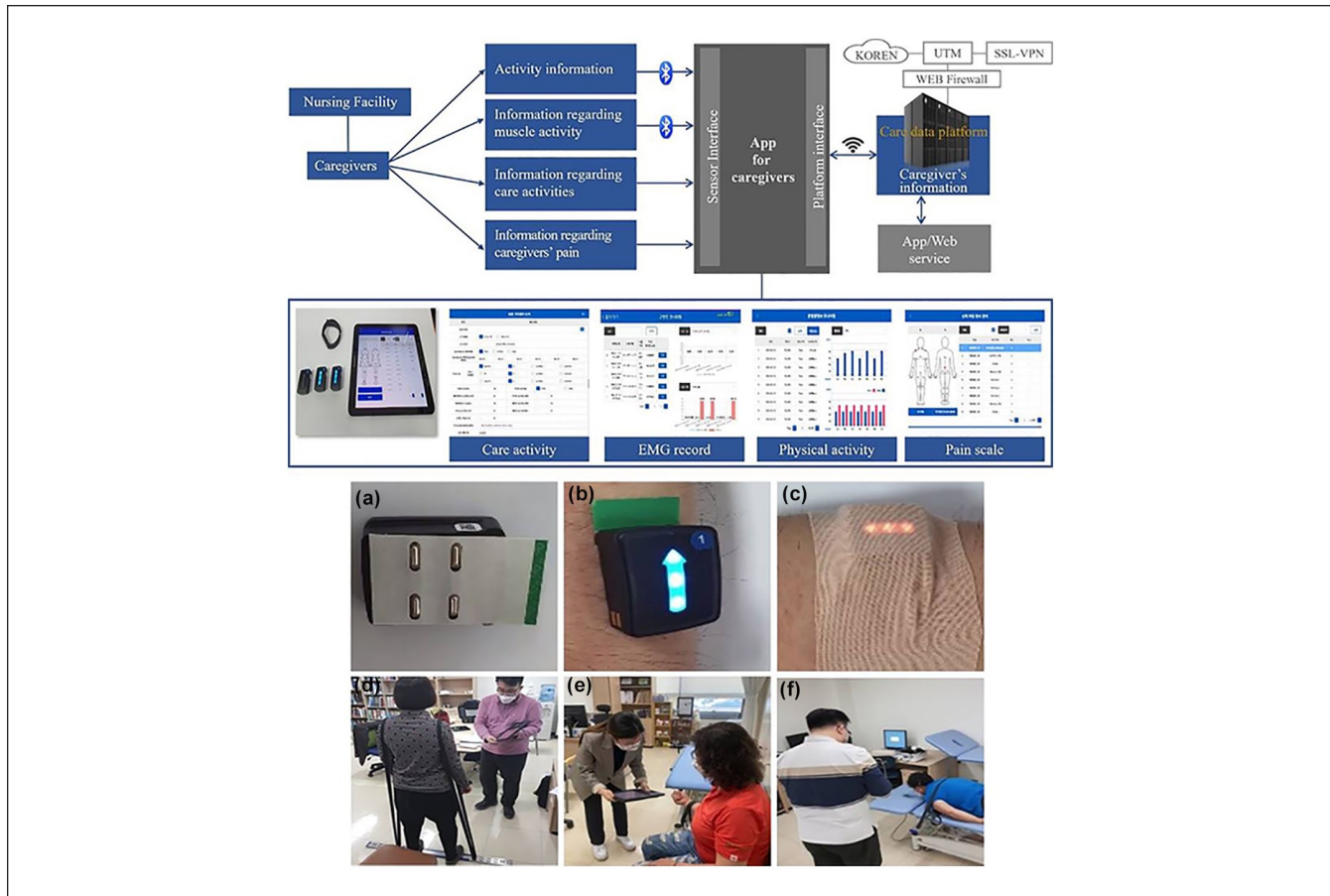
Figure 1. (Upper figure) Flowchart showing the study plan for caregivers' data collection and evaluation using the app): (a) Preparing a sensor and placing a gel patch, (b) attaching the sensor on the body, (c) applying elastic tapes to fix the sensor, (d) MVIC of the trapezius muscle (shoulder), (e) MVIC of the biceps brachii muscle (arm), (f) MVIC of the erector spinae muscle (back). MVIC = maximum voluntary isometric contraction.
