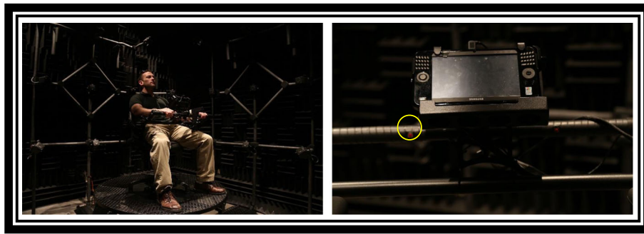
Fig. 1 Left panel depicts a listener seated in the center of the speaker array in the sphere room at the Environment for Auditory Research. The elevated platform allows for the listener to be centered within a ring of speakers positioned every 22.5°. The panel on the right depicts the micro PC used to present trial information to the participant. Participants responded using the red buttons mounted to the handle bar (positioned to the immediate left and right of the micro PC, highlighted in the yellow circles in the image at right)
