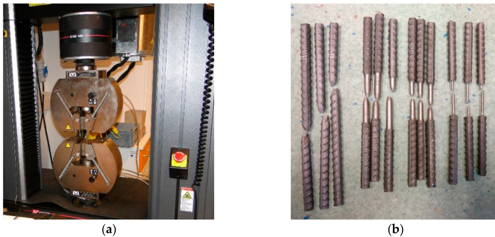
Figure 2. Test procedure: (a) Testing machine and (b) rebars.
