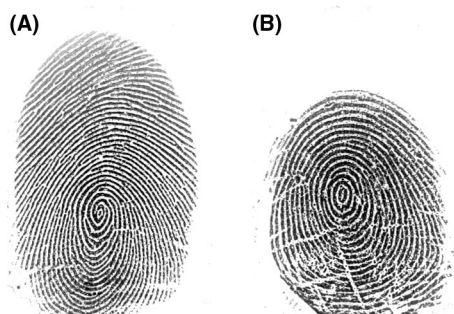
FIGURE 7 Images of hydrogel #1 (A) and hydrogel #2 (B) spoofs as acquired by device A. (optical)
