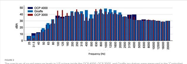
The spectrum of sound pressure levels in 1/3 octave inside the OCP 4000, OCP 3000, and Giraffe incubators were measured in the "Controlled environment room."
