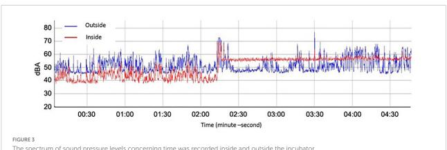
The spectrum of sound pressure levels concerning time was recorded inside and outside the incubator.
