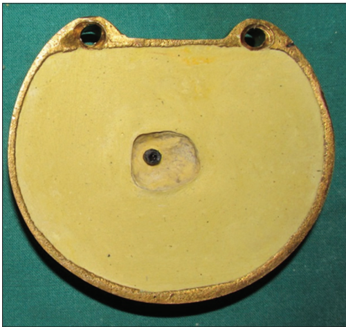
Figure 9: Upon dewaxing, removable cap is retained in the same position
