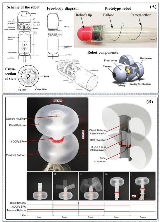
**Figure 5.** Examples of research-oriented innovative robotic colonoscopes and devices with pneumatic actuation: (**A**) self-steering pneumatically driven colonoscopy robot developed by Dehghani et al. [101]; (**B**) soft pneumatic inchworm double balloon (SPID) colonoscope developed by Manfredi et al. [102].
