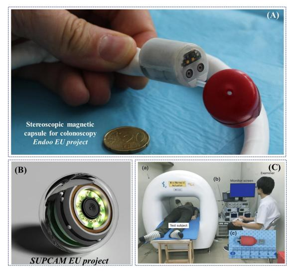
**Figure 6.** Examples of research-oriented innovative robotic colonoscopes and devices with magnetic or electromagnetic actuations: (**A**) Endoo EU project capsule (Courtesy of the Endoo consortium); (**B**) SUPCAM EU project spherical magnetic capsule for colonoscopy (Courtesy of Dr. Alessandro Tozzi); (**C**) modified PillCam<sup>TM</sup> SB2 with a silicone fin for magnetic locomotion through external electromagnetic fields, developed by Nouda et al. [128].
