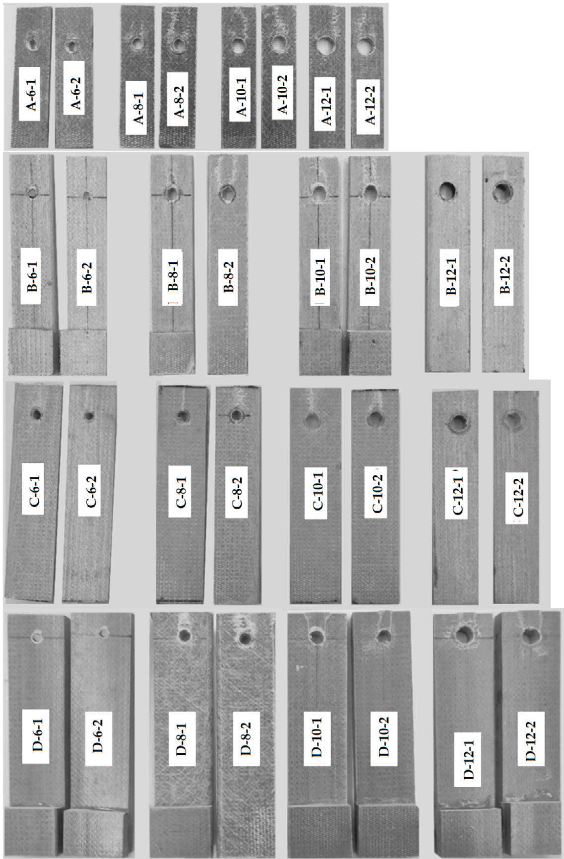
Figure 5. Failure patterns of the selected joints (scaled to represent actual size).
