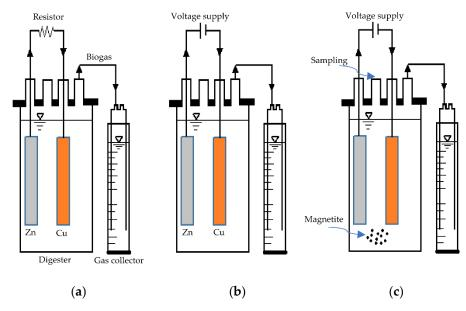
**Figure 1.** Schematic of anaerobic digestors: (**a**) microbial fuel cell (MFC); (**b**) microbial electrolysis cell (MEC); and (**c**) MEC with magnetite (MECM).
