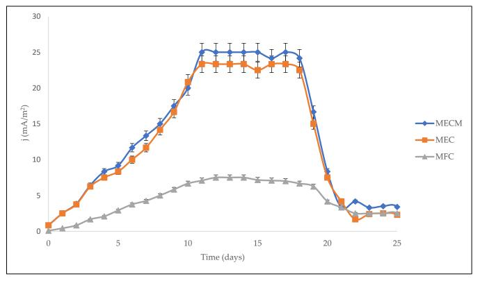
Figure 4. Effect of current density (j) on bioelectrochemical digesters.
