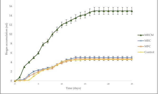
Figure 2. Biogas accumulation over the hydraulic retention time of 25 days.
