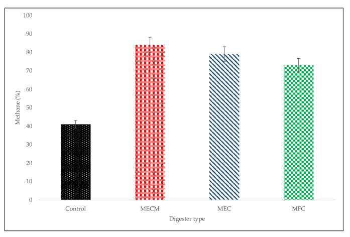
absolutely necessary for cytochromes and methane production [24,25]. The addition of Fe<sub>3</sub>O<sub>4</sub>-NPs in the MEC system promotes methane production by increasing the peak of the gas production and improving metalloenzymatic activities [25].
