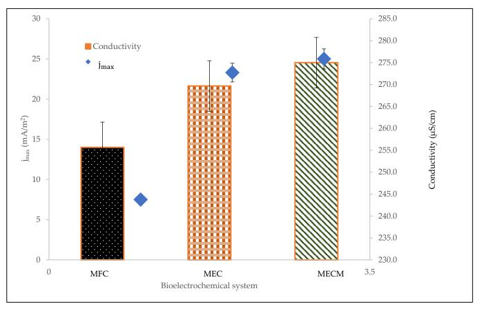
Figure 6. Effect of bioelectrochemical system on electrical conductivity.
