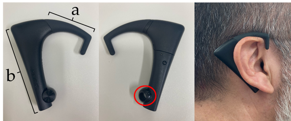
Figure 1. Ear-worn bite sensor (bitescan ® , Sharp Corporation, Sakai, Japan). (a) Variable ear hook; (b) body. The device is designed to be worn on the right side of the head. The lower part contains a sensor (circled in red).
