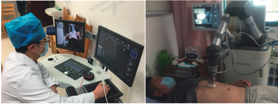
FIGURE 22: Remote ultrasonic inspection of 5G robots.
