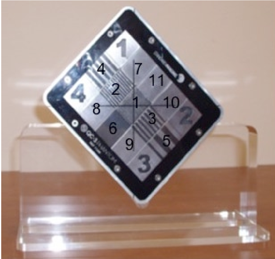
FIG. 3. QC-3 phantom with frame made up of aluminum and the sections made of lead and plastic.
