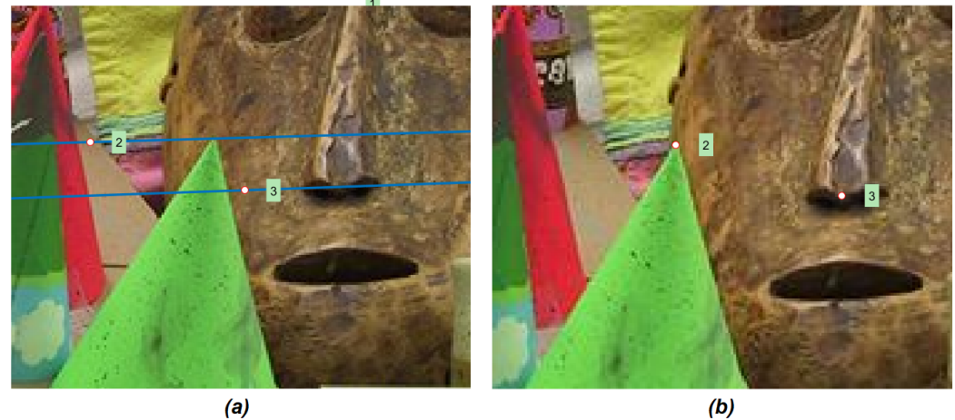
Figure 4. Details of the images shown in Figure 3. The tip of the cone (i.e., point number 2 in the image (b) depicting the right view I_R ) corresponds to a point that lies on the corresponding epipolar line (i.e., line number 2 in (a)) on the left view I_L .
