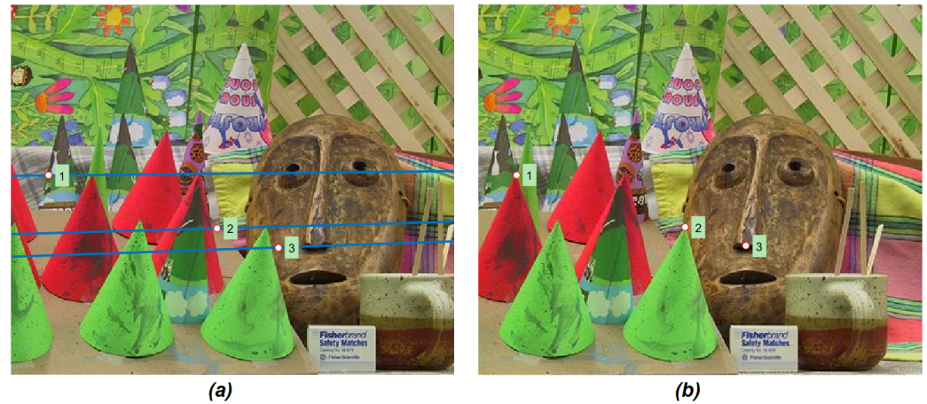
Figure 3. Considering any point in the right image (b) I_R (1, 2, and 3), the method in [20] searches the corresponding points in the left image I_L by computing their epipolar lines (a).
