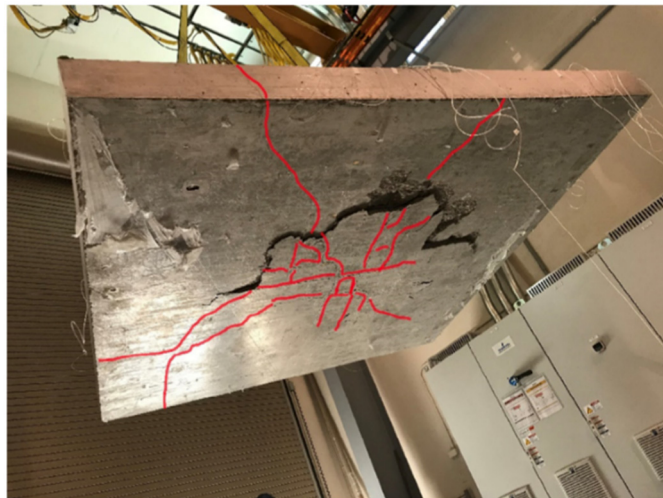
Figure 25. Specimen failure due to punching shear and its crack pattern [86].
