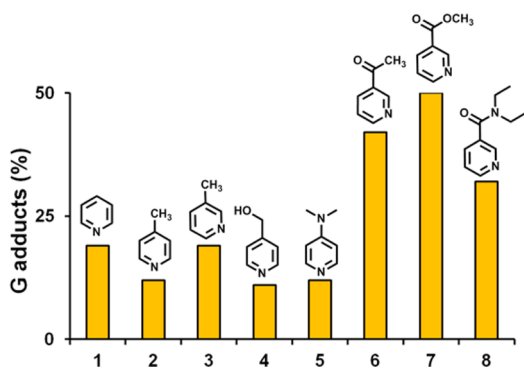
Figure 6. Bar chart showing the extent of binding of complexes 1–8 (ca. 1 mM in 20% MeOD- d_4 /80% D _2 O) to the nucleobase 9-EtG over 24 h at 310 K.
