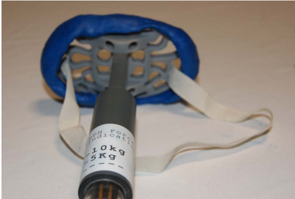
Figure 11 This iteration has a compression gauge as part of the central pillar supporting the platform (note the draft pulley system, designed to pivot the platform from a longitudinal position for insertion into a horizontal position for use).
