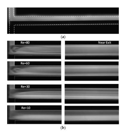
**Figure 7.** Planar mixing images obtained by experiment for (**a**) the simple T-mixer, Re = 80 and (**b**) the vortex micro T-mixer at different Reynolds numbers near the junction (left) and the exit of the mixing channel (right).
