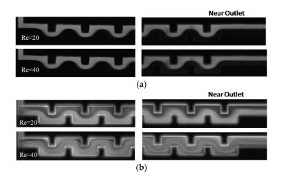
**Figure 10.** Experimental results. Micrographs for the intensity distribution in serpentine channels (at Re = 20 and 40) integrated with the (**a**) simple T-junction and (**b**) vortex T-junction. In the case of the serpentine channel with the simple T-mixer, the height of the channel is equal to the height of the inlet channels. In such a situation, the heights of the serpentine channel with the simple and vortex T-junctions are 100  $\mu$ m and 200  $\mu$ m, respectively.
