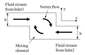
**Figure 1.** Basic schematic of the idea of vortex micro T-mixer. The two inlet channels of the vortex micro T-mixer are joining the mixing channel at an offset position. The height of the inlet channels is half the height of the mixing channel (h = H/2). The two fluid streams from Inlet 1 and Inlet 2 enter the channel at an offset position and create a vortex flow.
