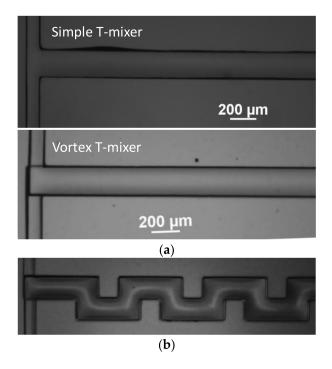
**Figure 3.** Micrographs of the experimental devices: (**a**) simple and vortex micro T-mixers and (**b**) planar serpentine channel integrated with vortex T-junction.
