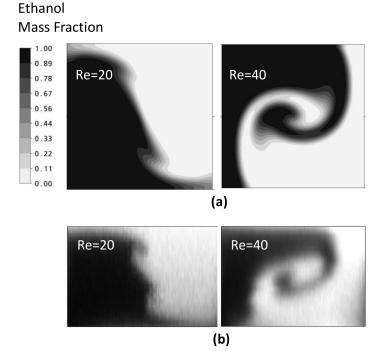
**Figure 5.** Comparison of the simulation and experimental results for the vortex micro T-mixer: (a) numerical results for the mass fraction distribution on y-z plane and (b) experimental results for the cross-sectional image [38].
