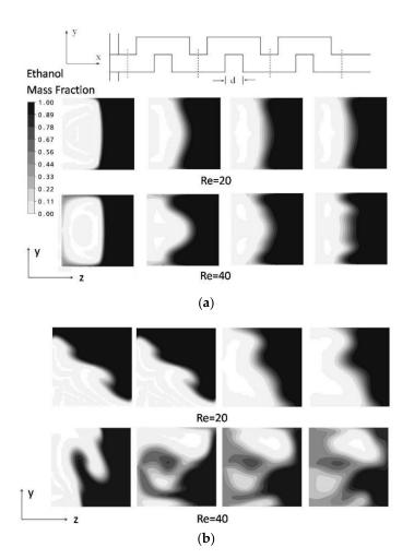
**Figure 9.** Mass fraction distributions of ethanol on the y-z planes at the initial four axial positions (shown by the dotted lines) in the planar serpentine channel at Re = 20 and 40 integrated with the (a) simple micro T-mixer and (b) vortex micro T-mixer.
