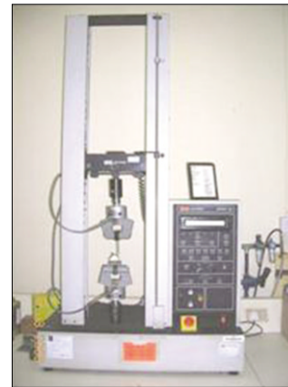
Fig. 4. Instron universal testing machine used.
