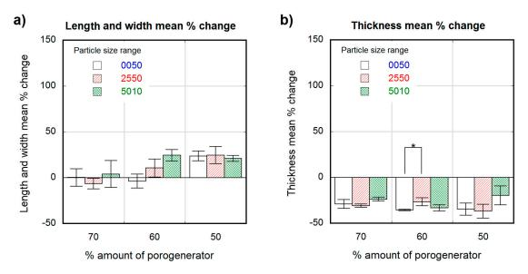
**Figure 4.** Dimensional variation in percentagevalues for dry scaffolds obtained from different particle sizes (white 0–50- $\mu$ m, stripe pattern 25–50- $\mu$ m, cross pattern 50–100- $\mu$ m) and proportions as a function of the theoretical percental amount of porogenerator: scaffold length and width mean % change (**a**); scaffold thickness mean % change (**b**). Significance level according to the Student *t*-test \* *p* < 0.05.
