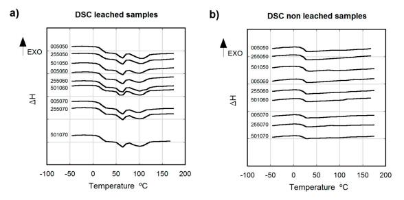
**Figure 5.** Thermograms of leached (**a**) and non-leached (**b**) aged samples (12 weeks at RT) produced using different porogenerator proportions and particles sizes (exothermic behavior upwards).
