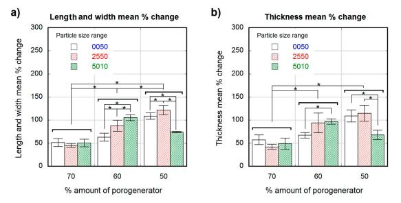
**Figure 3.** Dimensional variation in percental values for wet scaffolds obtained from different particle sizes (white 0–50- $\mu$ m, stripe pattern 25–50- $\mu$ m, cross pattern 50–100- $\mu$ m) and proportions as a function of the theoretical percental amount of porogenerator: Scaffold length and width mean % change (**a**); scaffold thickness mean % change (**b**). Significance level according to the Student *t*-test \* *p* < 0.05.
