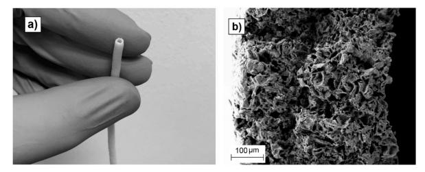
**Figure 8.** Tube with an inner diameter of 1.5-mm, a wall thickness of 400-µm, and a length of 300-mm produced by micro-extrusion (**a**); SEM image of a section of the tube wall (<500-µm) showing its porous structure (**b**).
