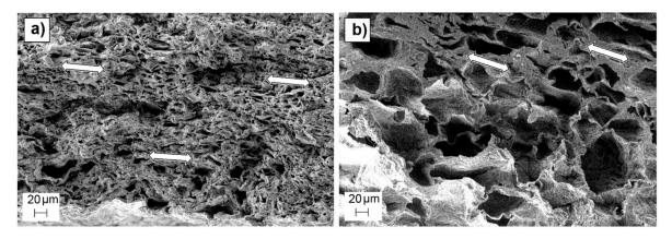
**Figure 7.** SEM images of cross-section surfaces of 005050 (**a**) and 501070 (**b**) scaffolds, showing the observed directional pore deformation highlighted by white arrows.
