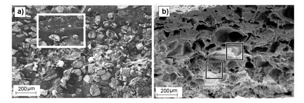
**Figure 6.** SEM images of cross-section surfaces of 501050 non-leached samples (**a**) and leached samples (**b**) showing non-porous polymer regions (outlined by a white rectangle in (**a**)) and remaining salt particles (outlined by squares in (**b**)).
