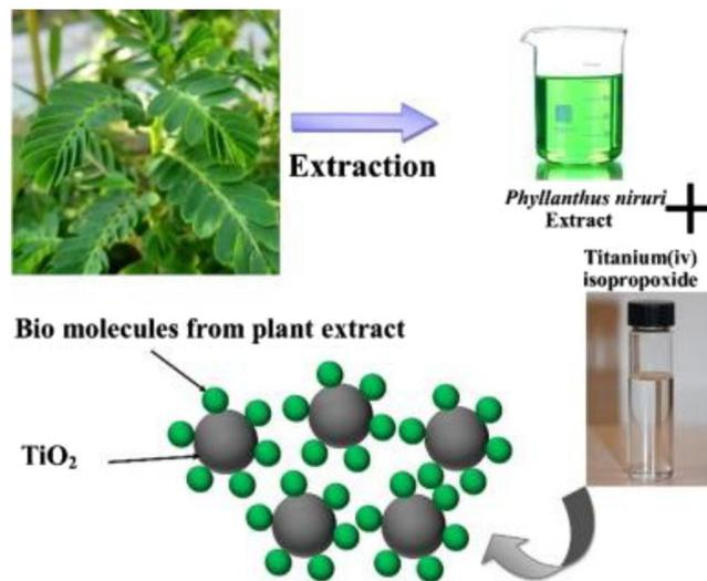
FIGURE 1 Green synthesis of TiO<sub>2</sub> nanoparticles
