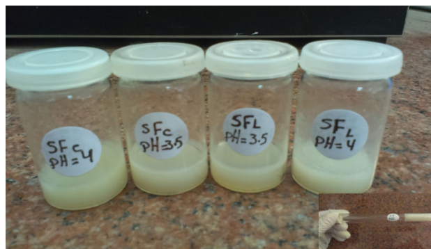
Fig. 2 Silk fibroin hydrogels at several pH values. The inset shows inverted test tube for following the gel development
