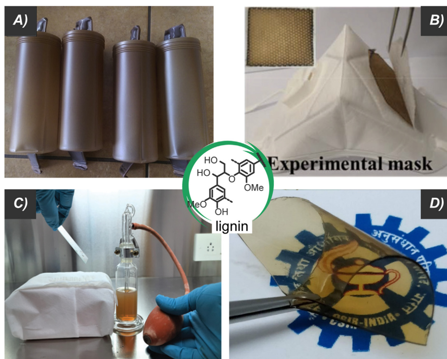
Fig. 13. A) Antimicrobial polyethylene container of capacity 500 cm 3 obtained from composite filled with 5% by weight of 1:5 wt/wt ZnO/lignin [335]. B) Antibacterial mask with amino acid-functionalized lignin in the inner filtering layer [229]. C) Lignin nanospray was coating onto the surface of a glass slice [336]. D) Digital images of gelatin/lignin antimicrobial package film [337].
