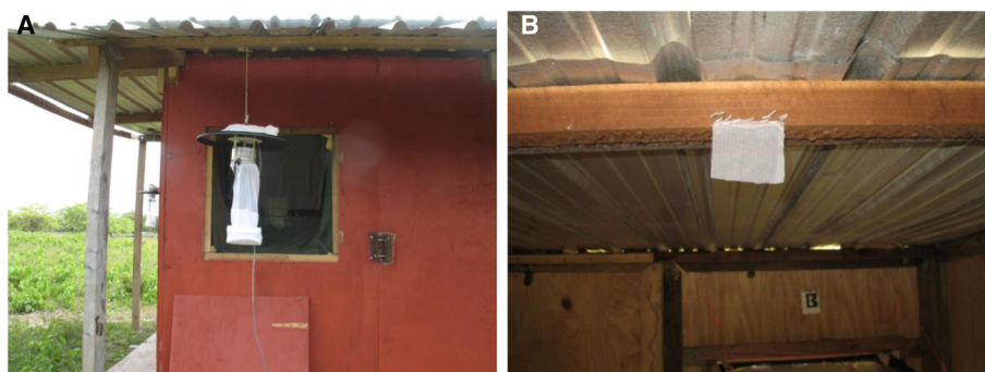
Figure 3 Experimental treatments. (A) An outdoor baited CDC light trap and (B) a spatial repellent emanator inside an experimental hut.
