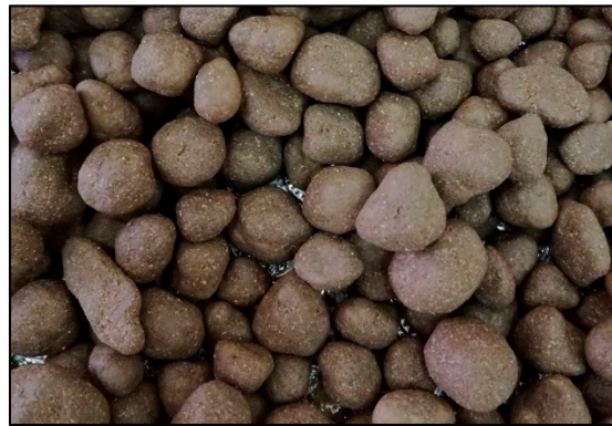
Figure 5. PCM impregnated LECA with geo-polymer coating.
