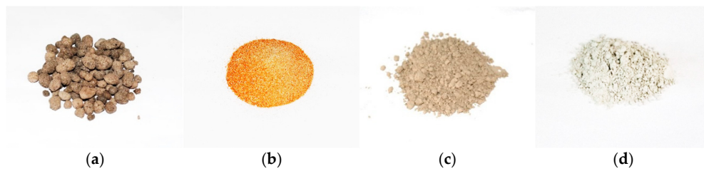
Figure 1. Photographs of (a) LECA, (b) DS, (c) FA, and (d) GGBS.
