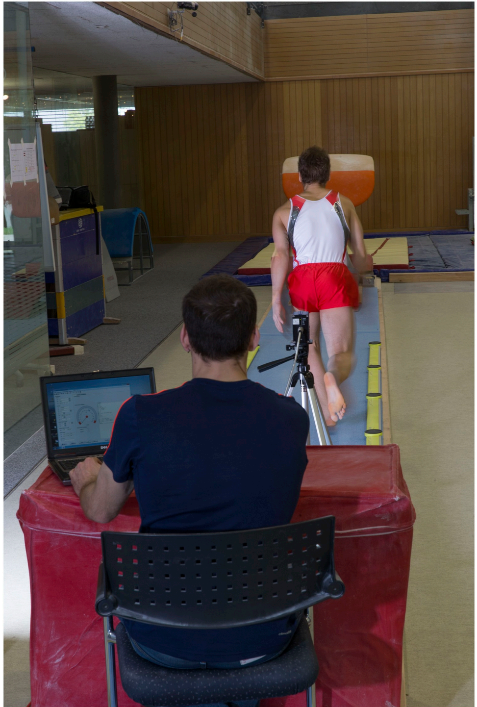
Fig 2. Experimental set-up. Measurement of maximal run-up speed (laser: LDM301a, Jenoptik, Rostock, Germany) and step kinematics (step frequency, step length, ground contact time) on vault (Opto Jump, Microgate, Italy). The individual in this figure has given written informed consent (as outlined in PLOS consent form) to publish these case details.
