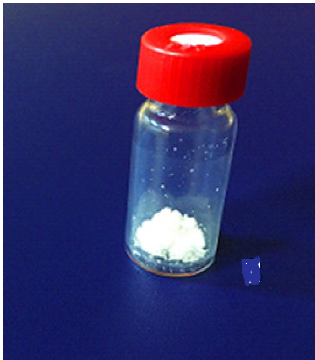
Figure 8. cPNIPAAM produced in emulsion of SC-CO 2 in water after lyophilizing.
