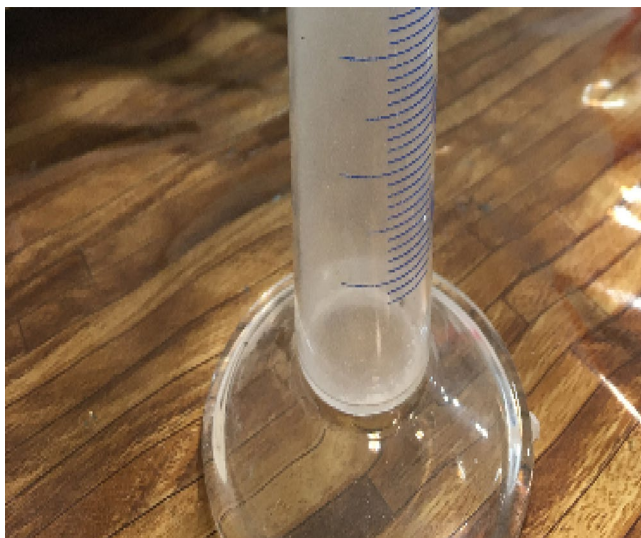
Figure 3. Residual raw materials, exited from the reactor by SC-CO 2 after depressurizing.
