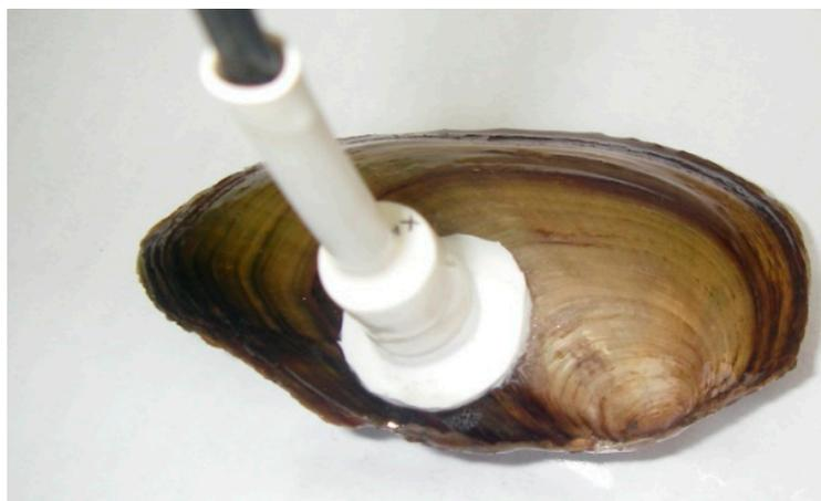
Figure 1. Sensor on the shell of *A. anatina* mussels.
