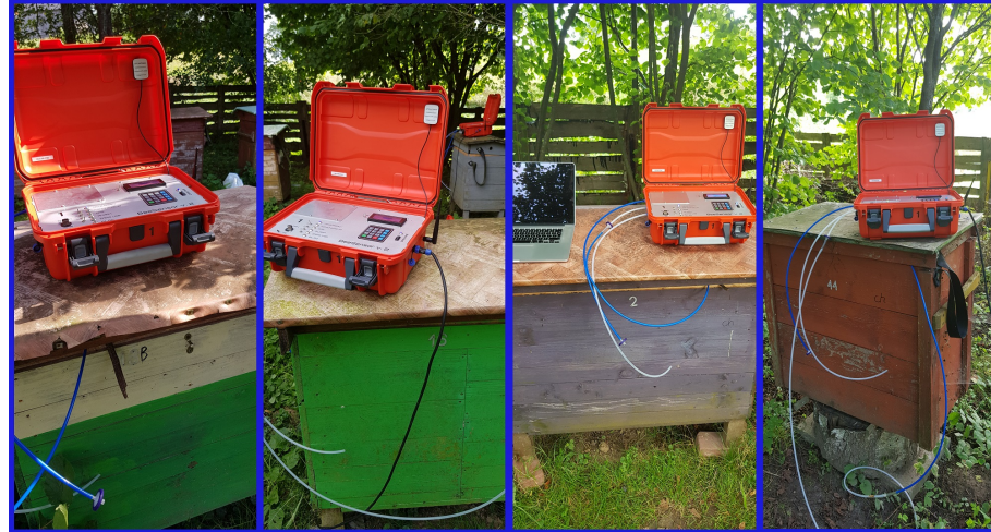
Figure 3. Multi-sensor recorder Beesensor V.2, unit BEECOM 1, during the measurement session of the different bee colonies.
