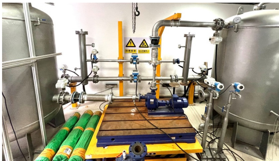
Figure 2. The experimental system for measuring the centrifugal pump efficiency.
