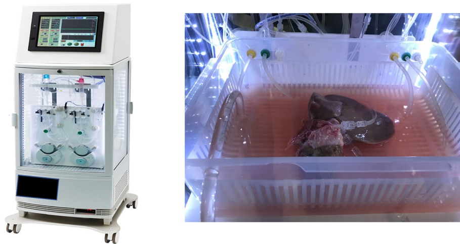
Figure 1. Perfusion preservation machine. The grafts were perfused using an originally developed MP system (CMP-X04W; Chuo Seiko Co., Ltd., Asahikawa, Japan).
