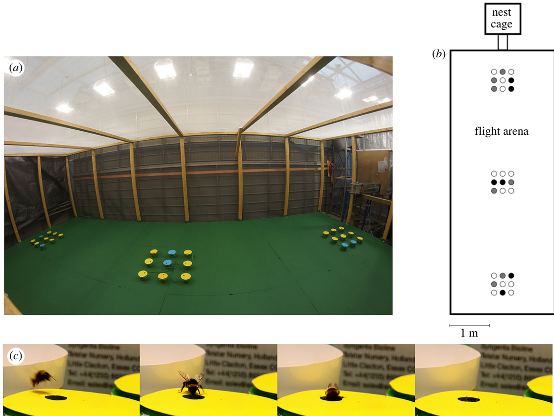
Figure 1. (a) Photograph and (b) schematic diagram of the experimental design of the flight arena used to quantify bumblebee foraging behaviour. Size of robotic flowers in (b) is only illustrative. White circles represent yellow (rewarding) flowers, while grey and black circles represent orange and blue (both punishing) flowers. (c) Time series photographs of foraging by a bumblebee on a robotic flower (during training in the nest cage). Photo (a) credit: Lassi Kalleinen; photo (c) credit: Kari Saikkonen.
