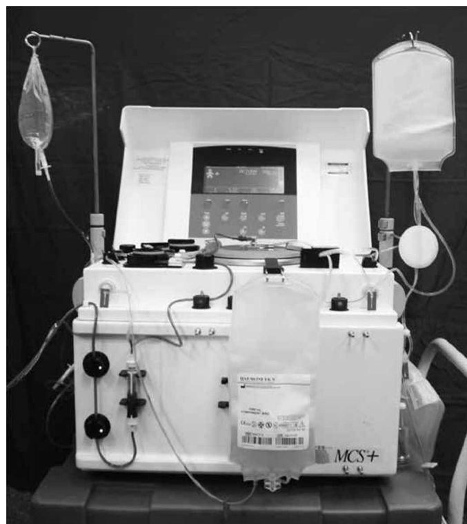
Figure 1 – Haemonetics MCS+ 9000 ® cell separator and 994-CFE apheresis-specific set (Haemonetics Corp., MA, USA).
