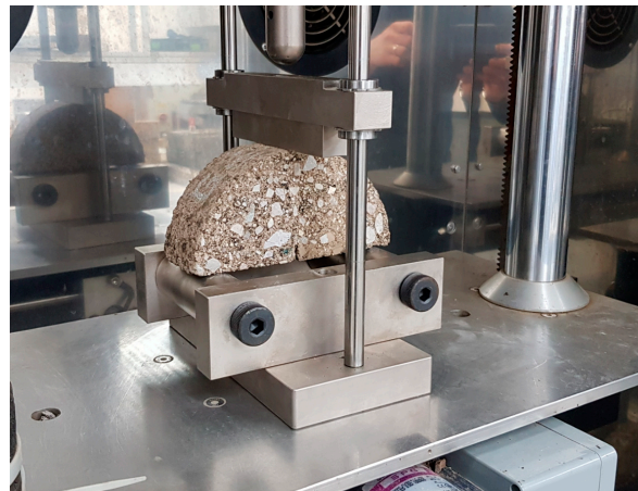
Figure 4. Semi-circular bending test set-up and specimen, fracture toughness test set-up (laboratory at Faculty of Civil Engineering and Architecture, Kielce University of Technology, Kielce, Poland) (source: M. Krasowski).
