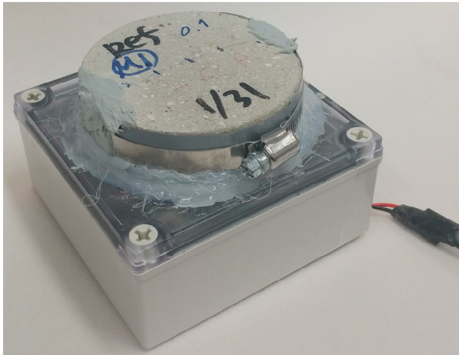
Figure 3. Mortar specimens attached on the airtight container.
