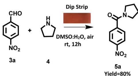
Scheme 7 Oxidation amidation of 4-nitrobenzaldehyde with pyrrolidine using dip strip of derivative C4 under visible irradiation at room temperature and aerial conditions.
