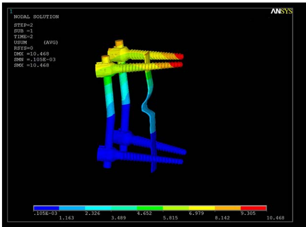
Figure 5. Strain in the pedicle internal fixation device and posterior longitudinal ligament under a 6mm extension displacement. The posterior longitudinal ligament displacement is not obvious.
