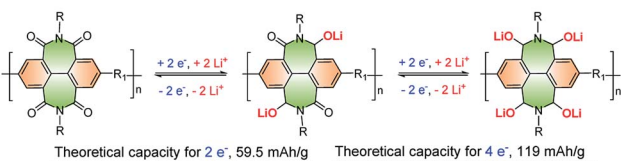
Scheme 1 Electrochemical lithiation and delithiation of representative polyimides and PBPI .
