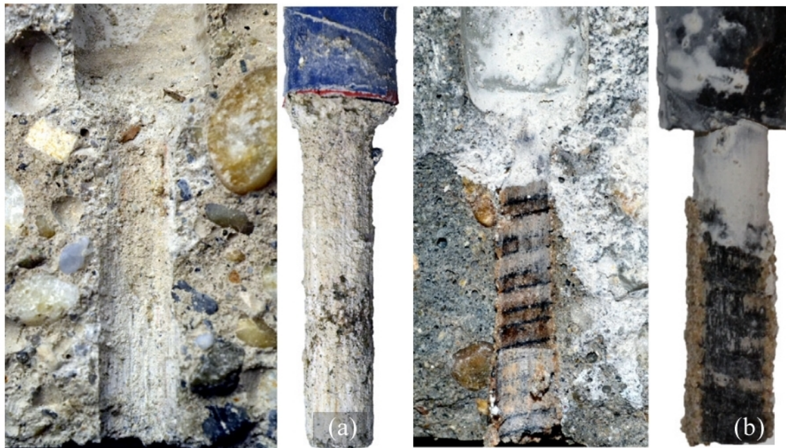
Figure 9. Failure types: (a) Concrete shear failure; (b) Peeling of rebar [36].
