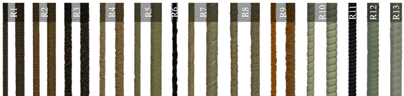
Figure 3. Surface deformation shapes of FRP rebars [58].
