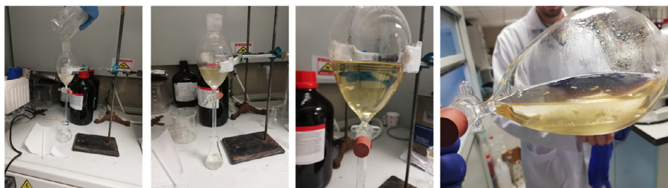
Fig. 3. Extraction with ethyl ether in separating funnel.
